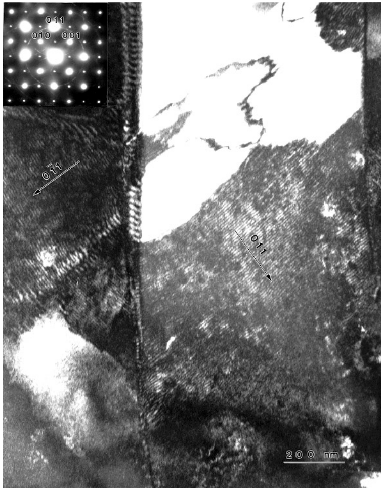
Figure 5. Dark-field image of a PZT06 ceramic obtained with the \frac{1}{2}(110)_p superlattice reflection.
