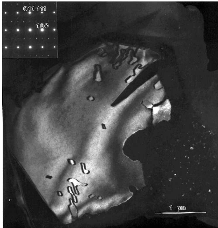
Figure 6. Dark-field image of a PZT12 ceramic obtained with the \frac{1}{2}(111)_p superlattice reflection.
